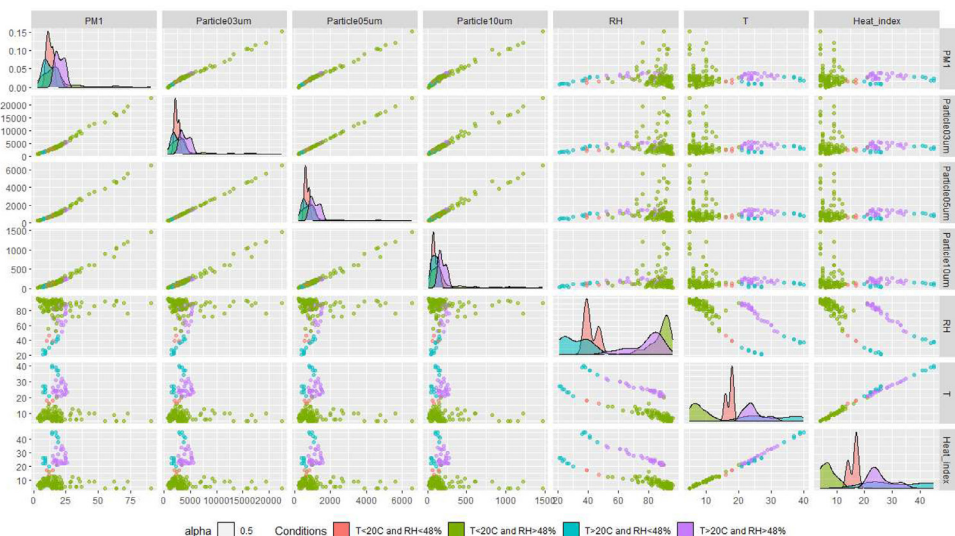
Fig. 2. Scatter and density plots were generated with the values recorded at the AQ-IoT-01 monitoring station and represent the association between the concentration of PM 1 (µg/m 3 ), particle sizes, and the meteorological variables measured by the PMS7003 low-cost sensor located in Reynosa, Mexico. Source: Author. Dataset: PM1_dataset_Average_Hour.csv.
