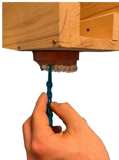
Figure 2. A specially built appliance was attached to the KaVo model to ensure standardized cleaning.
