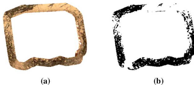
Figure 3. (a) shows the extracted photograph. (b) presents the black-and-white picture of the cleaned, white areas and the uncleaned, black areas.
