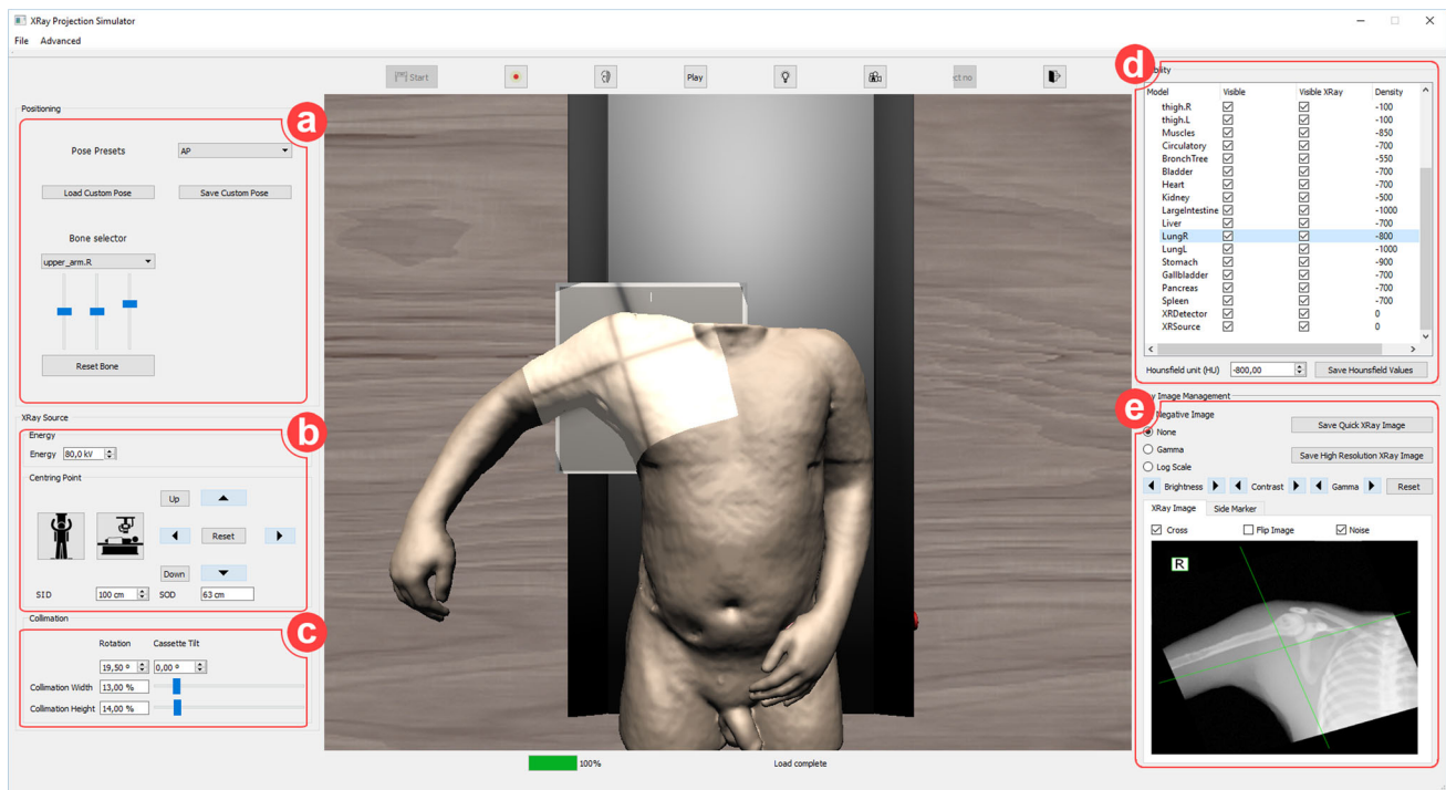
Fig. 1 GUI of the projectional radiography simulator: a patient positioning options, b centring, tube voltage, source-object distance and source-cassette distance configuration c collimation setup, d tissue visibility and material properties, e side marker's selection and digital image manipulation
