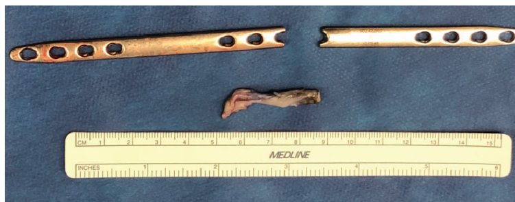
FIGURE 5: Damaged EPL and bridge plate. The excised portion of the frayed EPL tendon is photographed next to the broken dorsal spanning plate. This damaged portion of the EPL tendon was at the level of the broken plate in situ.
