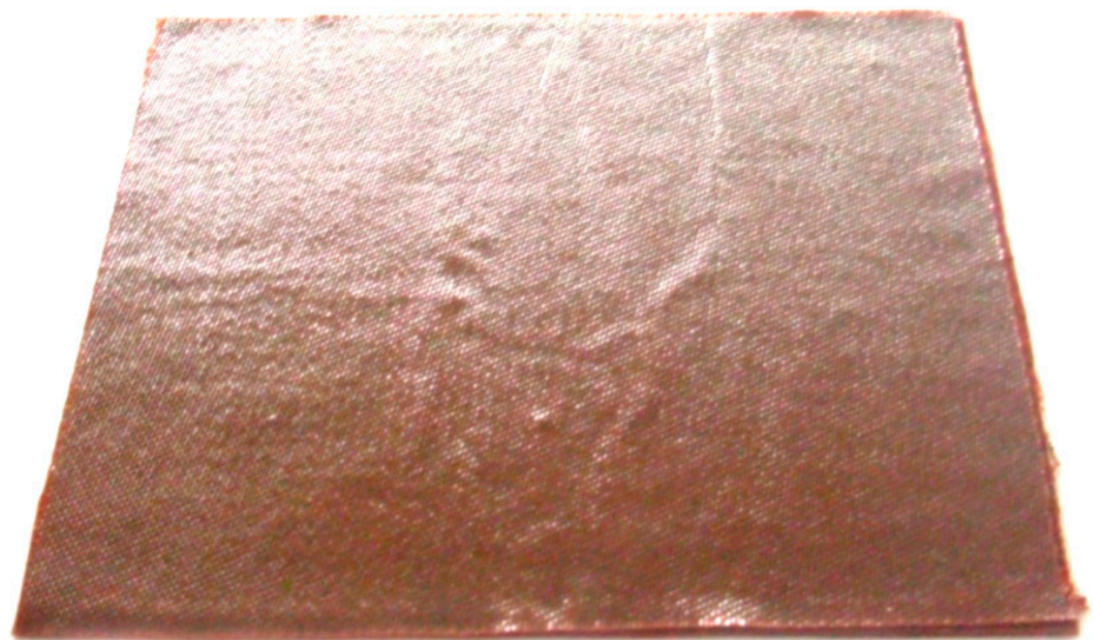
Figure 8. Upper surface of the specimen obtained with the use of moulding mode No 3.
