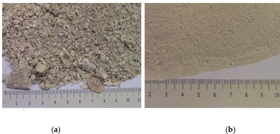
Figure 3. (a) Sample of white silicon dioxide before grinding; (b) Sample of the white silicon dioxide after pre-grinding in PM 400.
