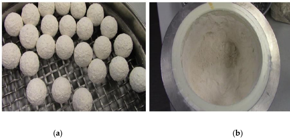
Figure 4. (a) Sample of white silicon dioxide before grinding; (b) Sample of the white silicon dioxide after pre-grinding in PM 400.
