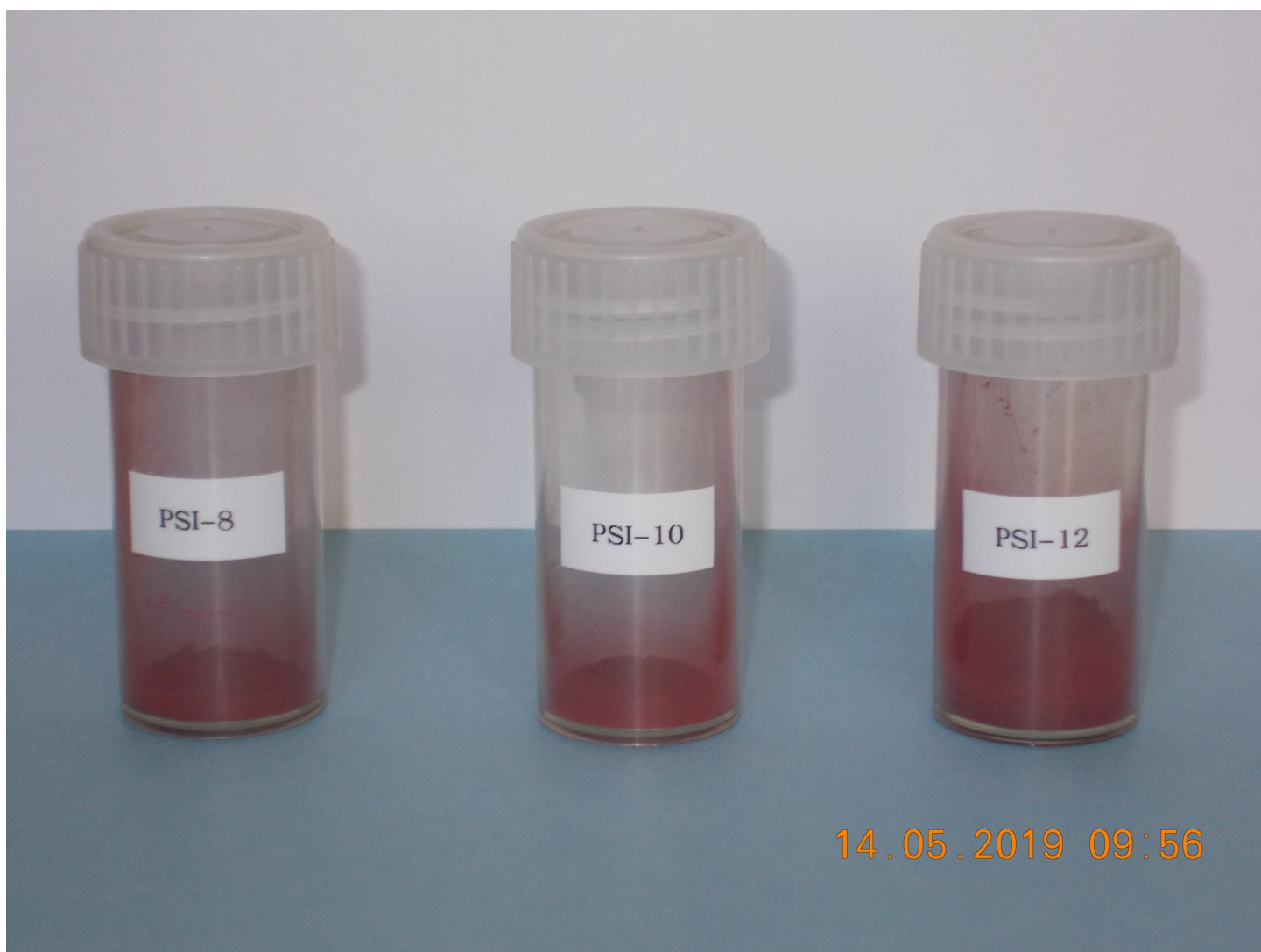
Fig 2. 60 Fe standard material as oxide powder (Fe 2 O 3 ). Around 1.6 g of PSI-8 and PSI-10, respectively, as well as around 16 g of PSI-12 were produced.
