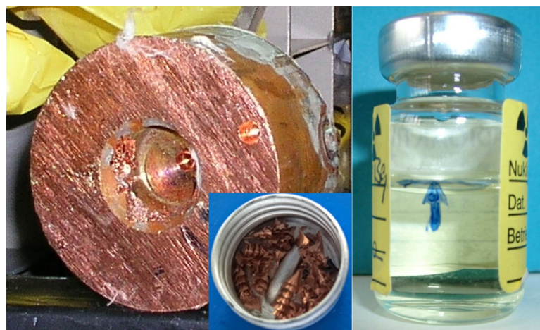
Fig 1. Left: Photography of piece 2 of the copper beam dump. The inset at the right bottom shows the chips drilled out at the central part. Right: Photography of the master solution. The blue arrow marked the initial level of liquid (5 ml) when used for the half-life measurement.
