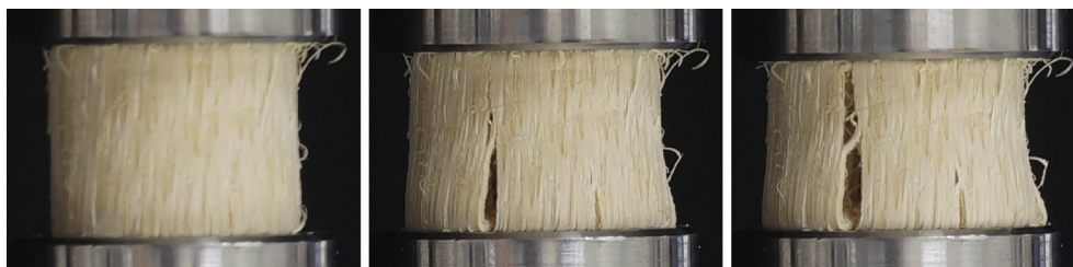
Fig. 23. A sequence of photos showing progressive failure (involving exfoliation by fiber buckling) of a rattan wood specimen during uniaxial compression.
