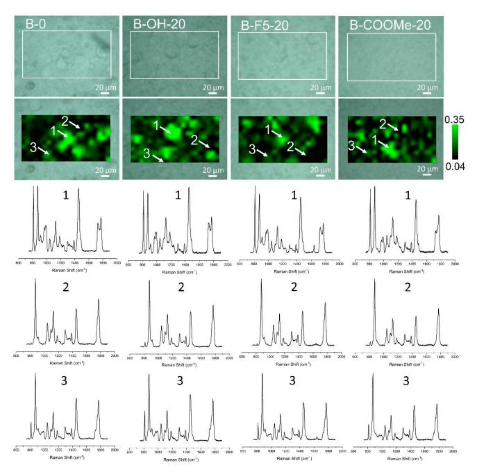
**Figure 7.** Raman maps of PLA/PMMA and ternary blends with 2 wt.% content of LPSQ-R illustrating distribution of PMMA in the blends (with corresponding optical micrographs in the background) and spectra of selected regions.
