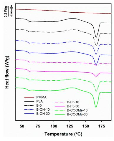
**Figure 8.** DSC thermograms of neat PLA, PMMA, PLA/PMMA and PLA/PMMA blends modified with LPSQ-R recorded during the second heating at  $5 \,^{\circ}$ C min<sup>-1</sup>.
