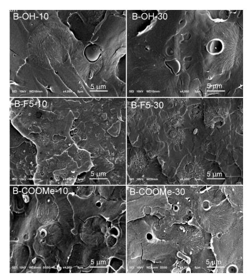
Figure 4. SEM micrographs of cryo-fracture surfaces of PLA/PMMA blends modified with LPSQ-R.
