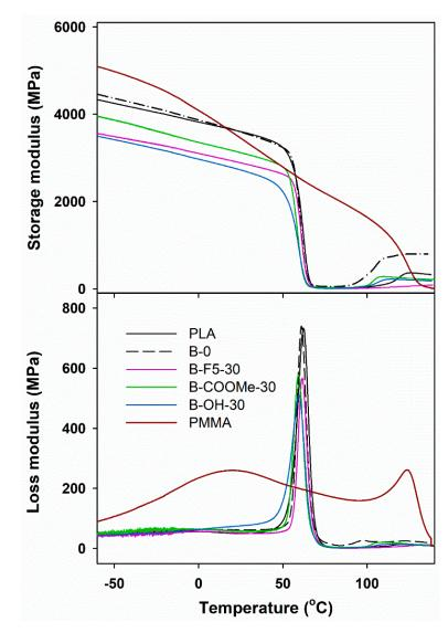
**Figure 1.** Storage modulus (*E'*) and loss modulus (*E''*) of neat polylactide (PLA), poly(methyl methacrylate (PMMA), PLA/PMMA blend (B-0) and selected LPSQ-R modified blends vs. temperature.
