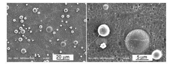
Figure 3. SEM micrographs of PLA/PMMA blend film etched for 1 h.
