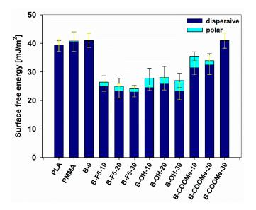
**Figure 12.** Changes of surface energy measured for native PLA, PMMA, their blend B-0 and blends with LPSO-R.
