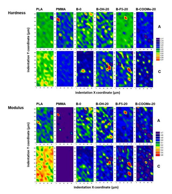
**Figure 11.** Maps of nanomechanical properties (hardness *H* and elastic modulus *E*) in compression moulded samples of the neat components and selected blends (A: surface area; C: cross-section, middle area).
