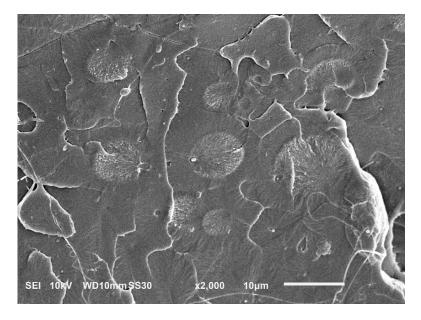
Figure 2. Scanning electron microscopy (SEM) micrograph of cryo-fracture surface of PLA/PMMA blend.
