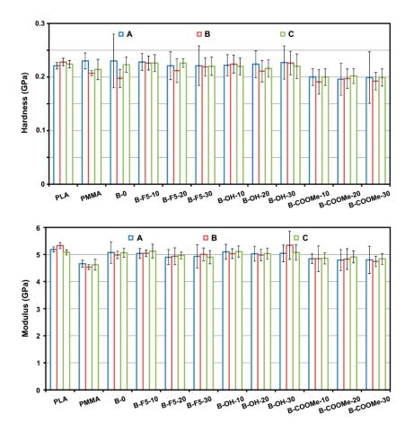
**Figure 10.** Average mechanical properties (hardness *H* and elastic modulus *E*) in the studied samples (A: along the surface B: cross-section at the edge; C: cross-section, middle area).
