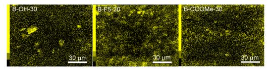
**Figure 5.** SEM EDS Si mapping of PLA/PMMA blends modified with LPSQ-R.
