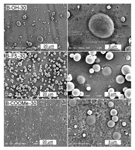
Figure 6. SEM micrographs of etched PLA/PMMA blends modified with 3 wt.% of LPSQ-R.
