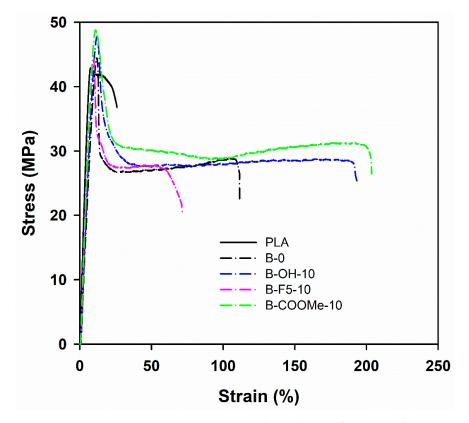
**Figure 9.** Engineering stress-engineering strain dependencies of PLA, PLA/PMMA and PLA/PMMA blend modified wit 1 wt.% of LPSQR, recorded during drawing at 5%/min.
