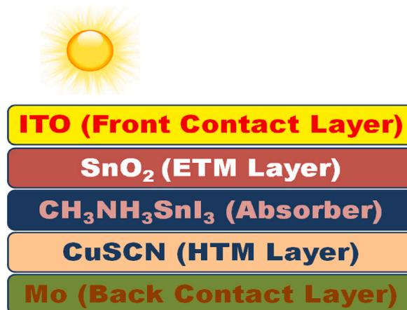
Fig. 1. Structure of proposed solar cell composition.
