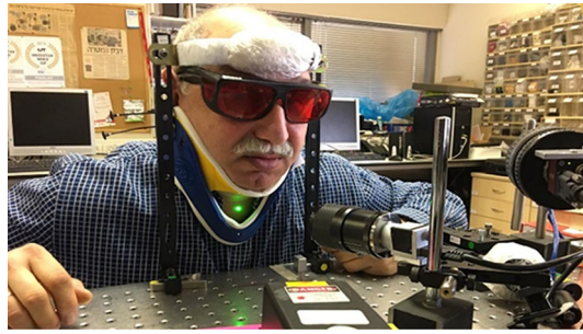
Figure 5. Setup of the system with its optics and the laser illuminating the neck of one subject.
