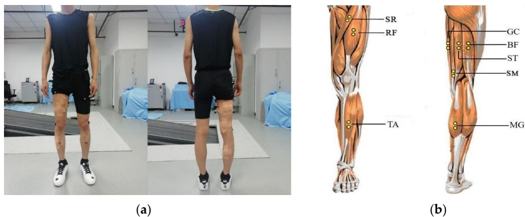
Figure 2. (a) Location diagram of sEMG sensors; (b) schematic diagram of human lower limb muscles used in this study.
