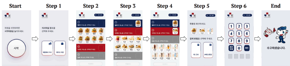
Fig. 2. Six sequential action steps in the virtual kiosk test between ‘Start’ and ‘End’ screens. In Step 1, the participants decide either to eat at the restaurant or to take out. In Step 2, participants select a burger. In Step 3, participants select a side. In Step 4, participants select a drink. In Step 5, participants select either to pay with cash or a credit card. In Step 6, participants enter the four-digit credit card password and then complete the order.
