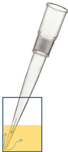
Figure 4. Position of pipette tips beneath liquid and in contact with the cross-sectional corners of the wells. Arrows indicate the flow of a cell suspension as the liquid is expelled, generating mild shear to disperse clumps and maximize mixing efficacy.
