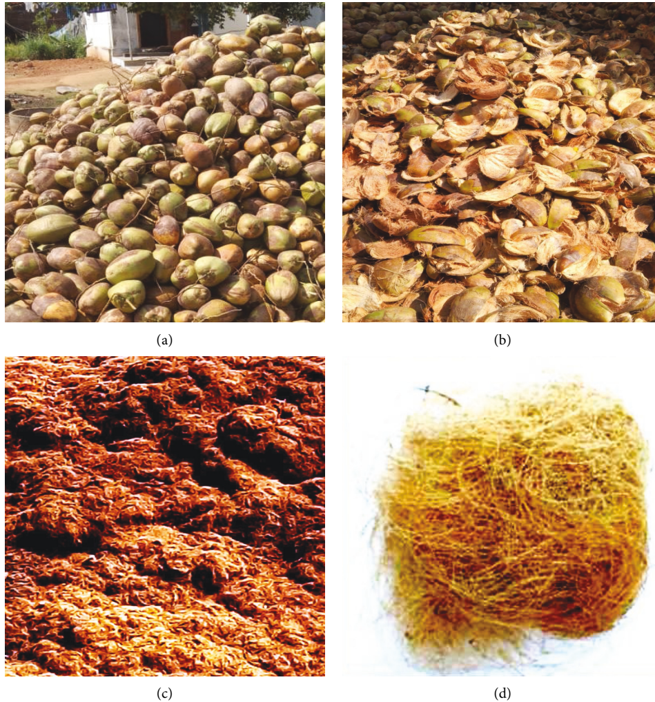
FIGURE 2: Schematic images of sample collection. (a) Primary husk. (b) Shells for backing support. (c) Areca husk fibre. (d) Coir fibre.
