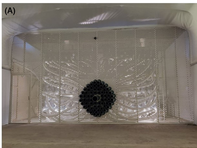
FIGURE 1 Immersive odor-presenting theater. (A) Electronically controlled olfactometer, Smell 2.0. (B) Spacious chamber in which the participants underwent immersive exposure to odors.
