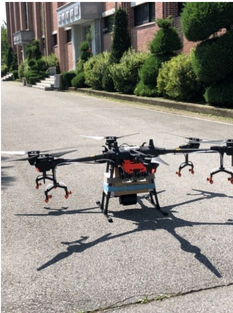
Figure 1 The drone used to transport the AED.
