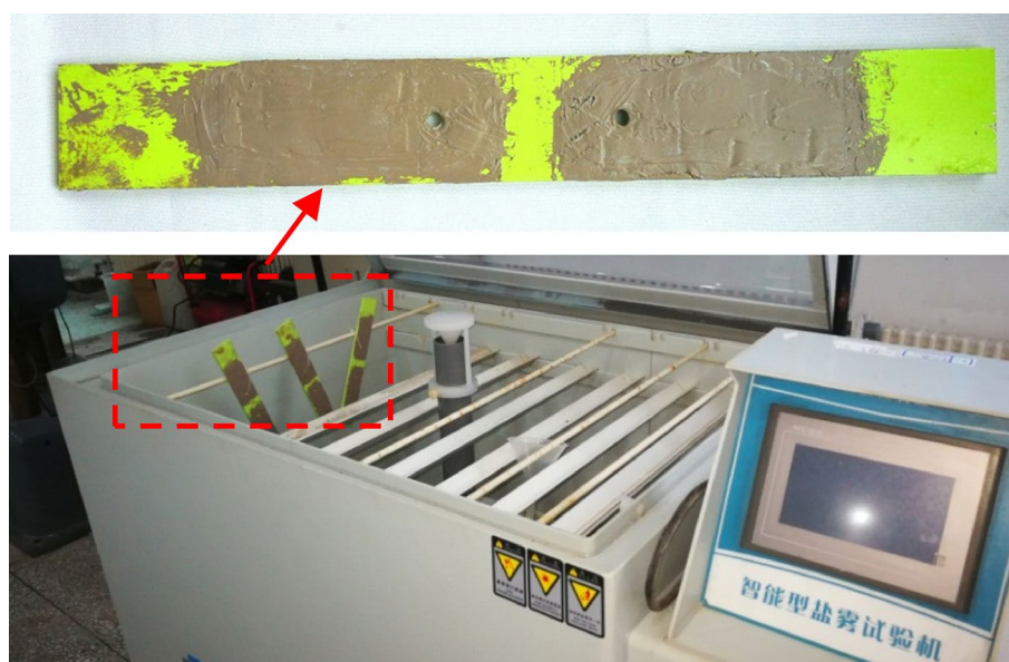
Figure 13. Salt fog corrosion experiment.
