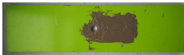
Figure 21. Surface of the specimen after Hygrothermal and ultraviolet radiation environmental experiment.
