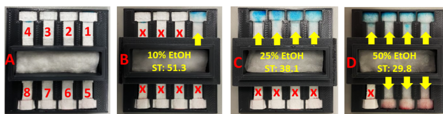
Figure 5. (A) Permeability-based surface tension measurement device. Modified papers in the channels have CWC of 6%, 12%, 17%, 22%, 36%, 42%, 49%, and 52% EtOH corresponding to positions 1 through 8, respectively. Applied aqueous EtOH solution concentrations: (B) 10%, (C) 25%, and (D) 50%, where ST stands for surface tension at 20 °C (mN m -1 ). Note: the papers used from positions 1 to 8 PAC(1), PAC(1.2), C4(0.8), POAC(1.2), C6(0.6), C6(1), C16(0.7), and C12(1) were modified at 80 °C for 6 h.
