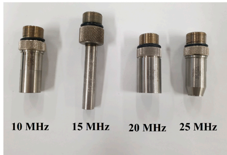
Figure 10. Transducer probes with each different frequency band used to measure the echo signals.
