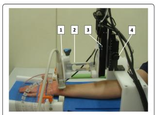
**Fig. 1** Setup for strain and pressure measurement. The participants were asked to sit and place their forearm on a table with the palmar side up. 1. Transducer holder, 2. Pressure sensor, 3. Motor for the compression-release cycle, 4. Placement adjuster
