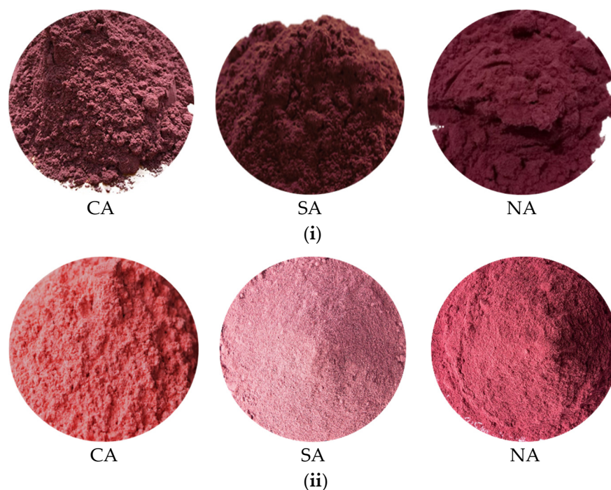
Figure 2. Images of pectin samples extracted from Fetească Neagră and Rară Neagră grape pomace under the influence of acid type: CA—citric acid, SA—sulfuric acid, and NA—nitric acid (fixed extraction conditions: particle size of \geq 125 – < 200 \mu\text{m} , at pH 2, 90 °C for 3 h). (i) Pectin samples extracted from Fetească Neagră grape pomace under the influence of acid type. (ii) Pectin samples extracted from Rară Neagră grape pomace under the influence of acid type.
