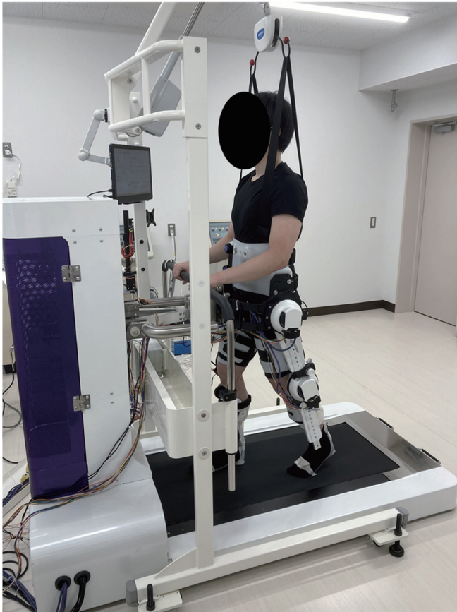
Fig. 1. Gait rehabilitation robot for paraplegia. The robot contains a functional electrical stimulation system for quadriceps femoris muscle and hamstrings of both sides, a treadmill, and a safety rehabilitation lift for unloading.
