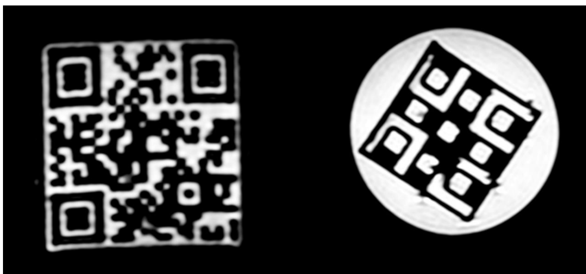
Figure 3. Representative coronal MR images of 3D printed phantoms. The left is the large QR cube, and the right is the Hilbert cube. The interested readers can read the presented QR code MR image using their smartphone's QR code reader.
