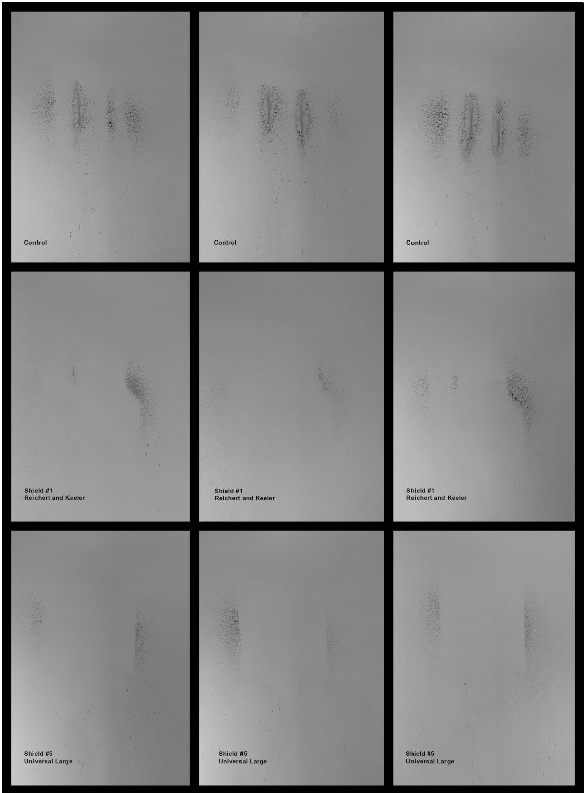
FIGURE 2. Sample overspray patterns from control (top), a breath shield attached to the objective lens arm (1, Reichert and Keeler style, middle row), and a breath shield hung by the oculars (5, Universal Large, bottom row).
