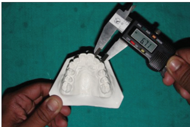
Figure 2: Digital Vernier caliper to measure the mesiodistal width of teeth
