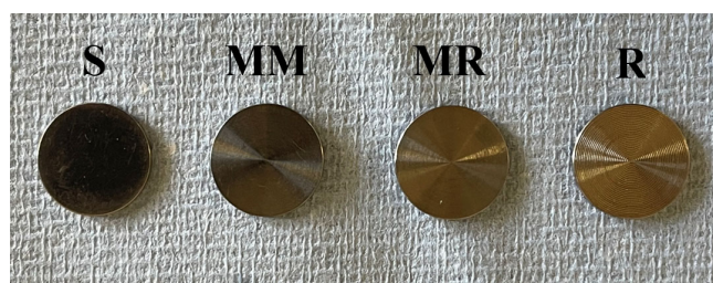
Figure 1. Ti discs with different roughness degrees (S, MM, MR, and R).
