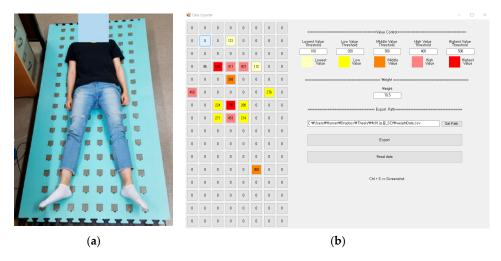
Figure 3. The lying posture in the smart mat (a) and the pressure distribution (b).
