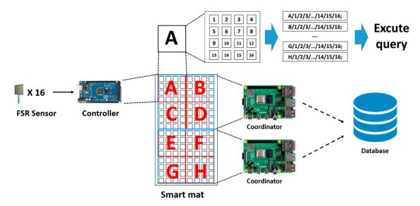
Figure 2. The hardware architecture of the smart mat system.
