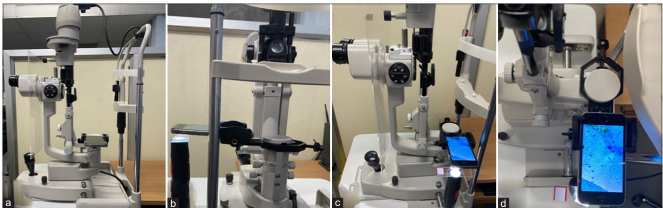
Figure 3: (a) Lateral view of SLIM assembly with a different slit lamp model; (b) View from patient's perspective of SLIM; (c) Lateral view of SLIM being used to image a slide; (d) Superior view of SLIM being used to image a slide
