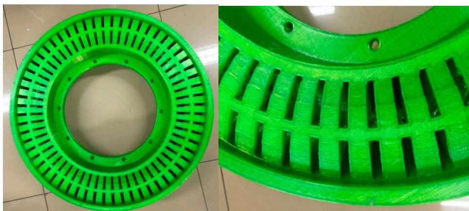
Figure 12. 3D printed non-pneumatic tire based on TPU material.
