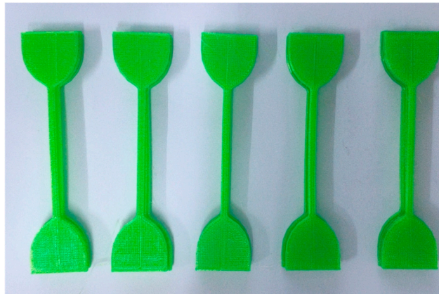
Figure 2. Dumbbell-shaped TPU specimens 3D printed by FDM technology.
