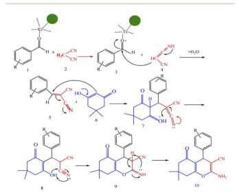
Scheme 1 A plausible mechanism for synthesis of chromens in the presence of nano-cellulose/ ${\rm Ti}^{\rm (IV)}/{\rm Fe_3O_4}.$
