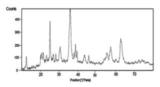
Fig. 2 XRD patterns of nano-cellulose/Ti<sup>(IV)</sup>/Fe<sub>3</sub>O<sub>4</sub>.
