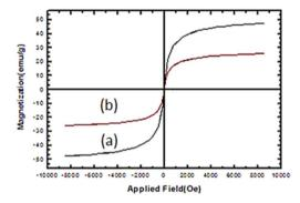
Fig. 6 VSM images of (a) Fe<sub>3</sub>O<sub>4</sub> and (b) nano-cellulose/Ti<sup>(IV)</sup>/Fe<sub>3</sub>O<sub>4</sub>.
