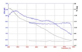
Fig. 5 Thermal gravimetric analysis pattern of nano-cellulose/Ti  $^{(\rm IV)}/$  Fe $_3{\rm O}_4$  catalyst.
