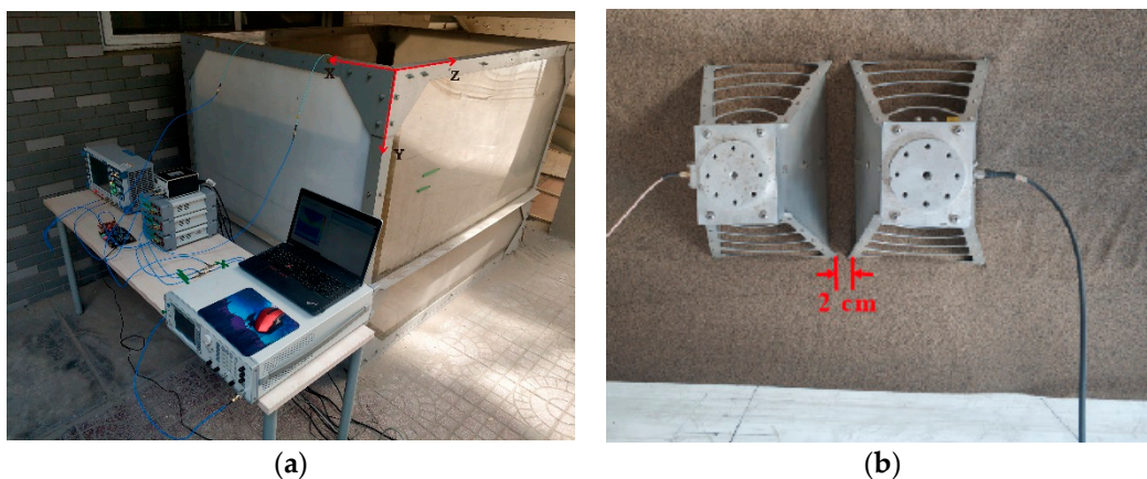
Figure 4. (a) The experimental scene of underground pipe location. (b) A photograph of the experimental tests in the sand container.
