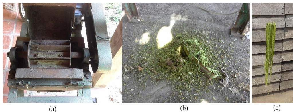
Figure 2. Curaua fiber extraction. (a) Machine used to separate fiber from leaves. (b) Mucilage residue after fiber extraction. (c) Curaua fiber drying in the sun.
