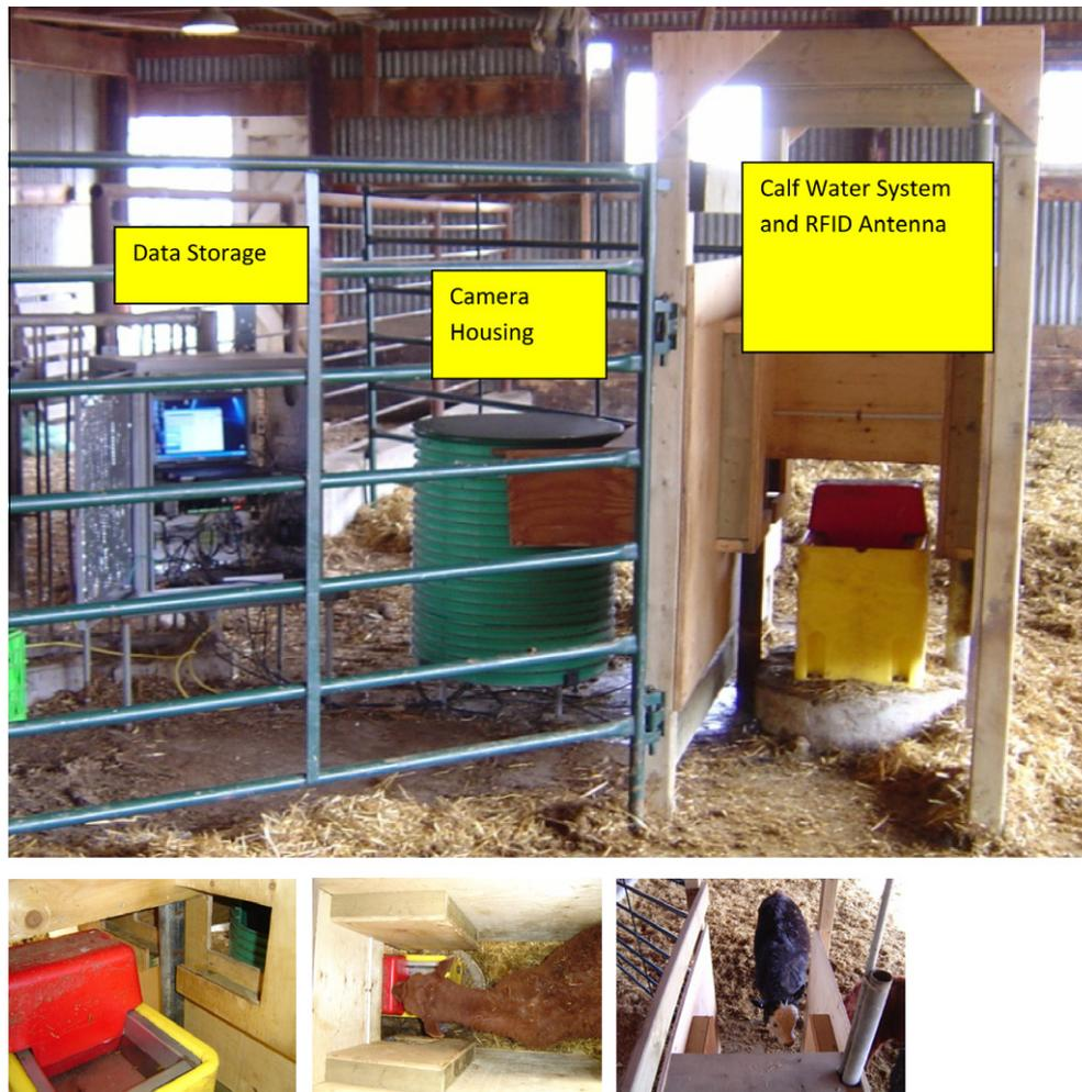
Fig. 1. Image of automated, RFID driven, non-invasive IRT scanning station located in a feedlot pen around a water station.
