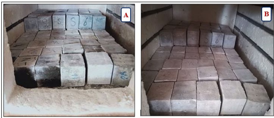
Figure 10. Concrete samples before (A) and after (B) 500 °C fire exposure.
