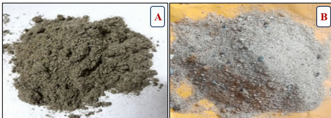
Figure 2. Used fine aggregate: (A) Black Sand and (B) Normal Sand [41].
