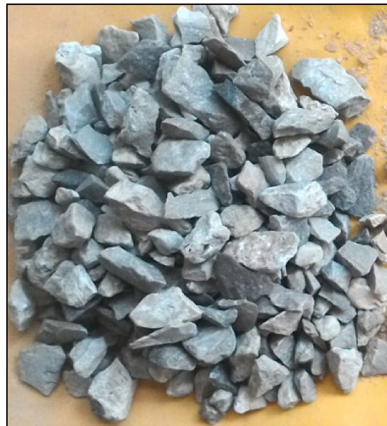
Figure 6. Used Crushed Dolomite.
