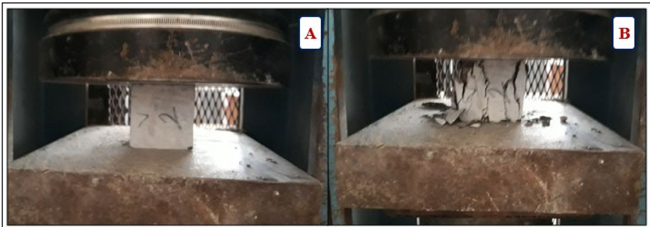
Figure 9. Compressive strength test: (A) test setup, (B) specimen failure.
