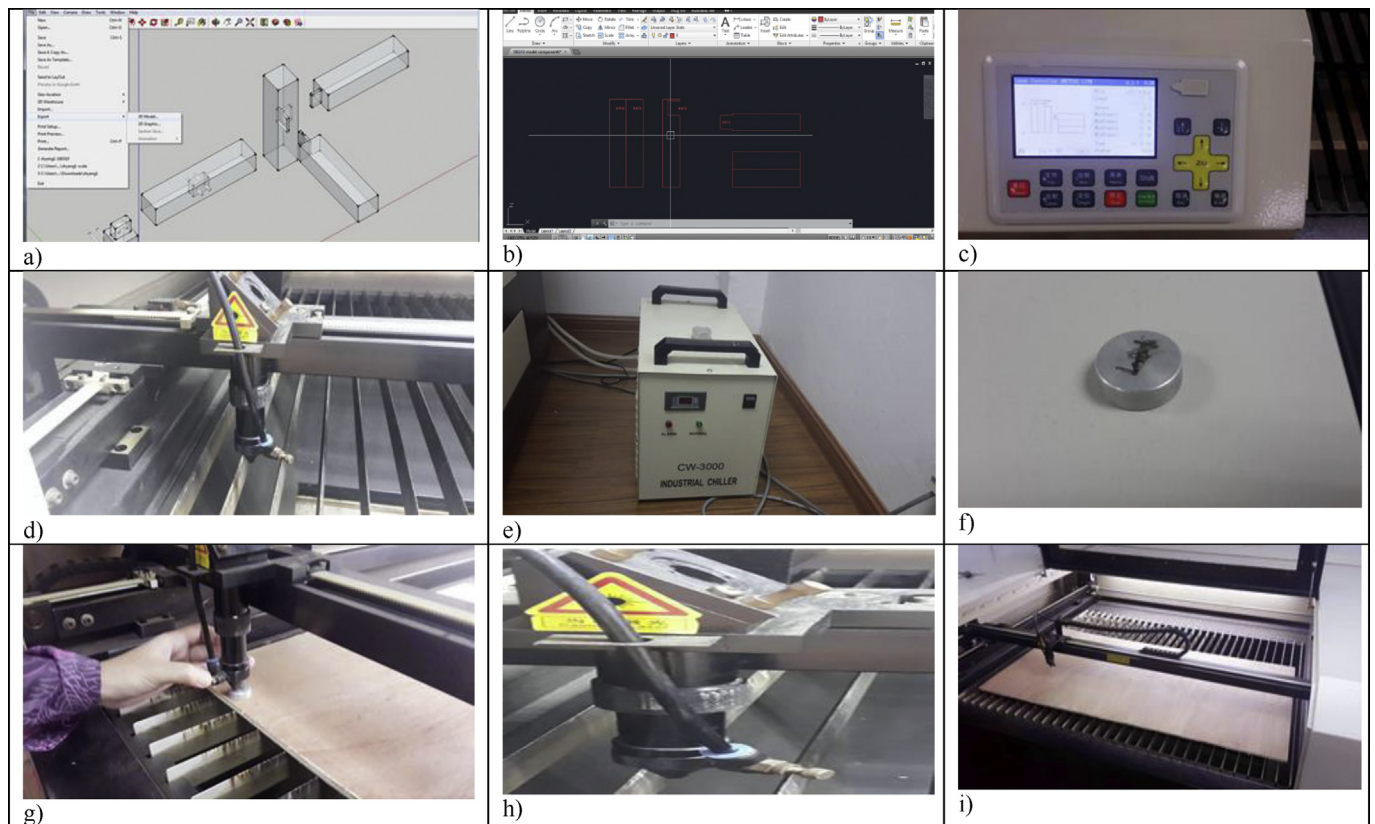
Figure 5. Set up apparatus for Laser Cutting: a) Export as .dxf file; b) Check the file with AutoCAD; c) Send the image to laser cutter; d) Lens cleaning; e) Chiller; f) Round metal for laser head; g) Setting laser head height; h) Blower; and i) Air cut.
