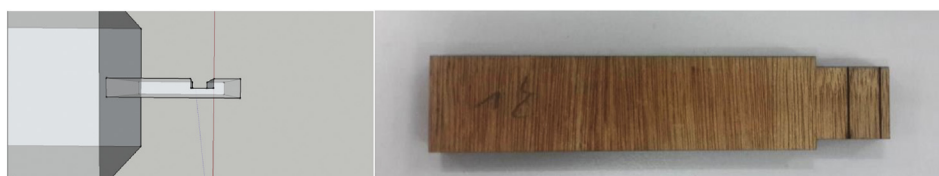
Figure 9. Concave part of hybrid mortise & tenon joint combining blind, interlocking, and angled in Model 4.
