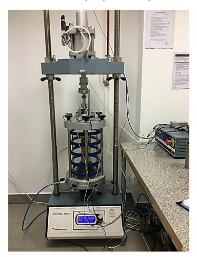
**Figure 5.** View of the cyclic triaxial apparatus with the sample in a cell before starting the test.
