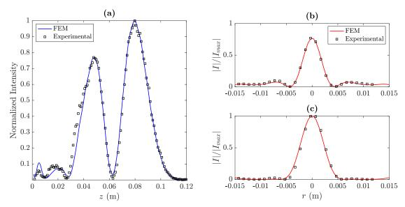
**Figure 7.** (a) Measured (black squares) and simulated (blue line) focusing profiles (longitudinal cuts) for the manufactured BiFZP lens. (b,c) Measured (black squares) and simulated (red lines) transversal cuts at  $z = F'_1$  (b) and  $z = F'_2$  (c).
