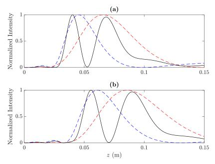
**Figure 3.** (a) The BiFZP focusing profile designed for  $F'_1 = 40$  mm and  $F'_2 = 68$  mm, and (b) the BiFZP focusing profile designed for  $F'_1 = 56$  mm and  $F'_2 = 90$  mm. In both cases,  $f_0 = 250$  kHz.
