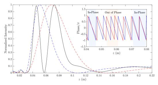
**Figure 2.** The bi-Fresnel zone plate focusing profile (black) compared to the inner (blue) and outer (red) focusing profiles. The phase of the inner (blue) and outer (red) profiles are shown in the inset.
