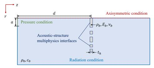
Figure 4. Scheme of the finite element method (FEM) model.
