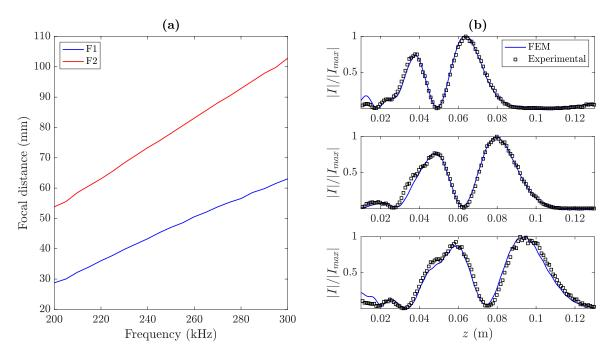
**Figure 8.** (a) BiFZP focal distance for  $F'_1$  (blue) and  $F'_2$  (red) as a function of the operating frequency and (b) BiFZP focusing profiles at 220 kHZ (top), 250 kHz (middle) and 280 kHz (bottom).
