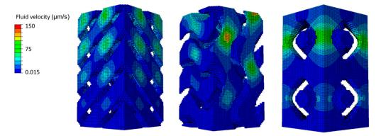
**Figure 5.** Fluid flow velocity distribution at peak compression over the collagen substrate in contact with TPMS scaffolds (left: SD70; center: SG70; right: SP70). Please note that the scaffold has been removed for the sake of visualization.
