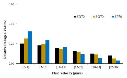
**Figure 6.** Fluid flow velocity distribution ( $\mu$ m/s) in the collagen substrate elements versus their relative volume, at peak compression, for the three FE models.
