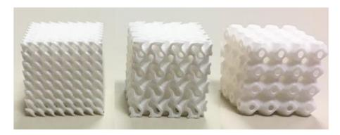
**Figure 1.** 3D printed scaffolds: Schwartz D (SD70), Gyroid (SG70), and Schwartz P (SP70) (from left to right).
