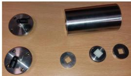
**Figure 2.** Experimental apparatus for the permeability tests (left: overview; right: permeability chamber parts).
