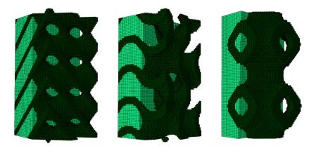
**Figure 3.** Finite element (FE) models of triply periodic minimal surface (TPMS) scaffolds embedded in 0.20% collagen substrate (left: SD70; center: SG70; right: SP70). Please note that dark green represents the scaffold and light green the collagen substrate.
