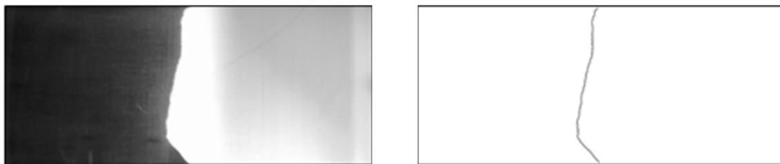
Figure 2. Instantaneous image of resin flow before and after image processing.
