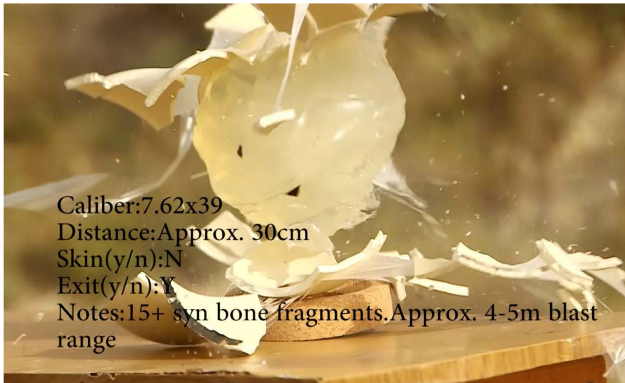
Fig. 2 Hydraulic burst of a Synbone® sphere at 30 cm with a 7.62 \times 39 mm
