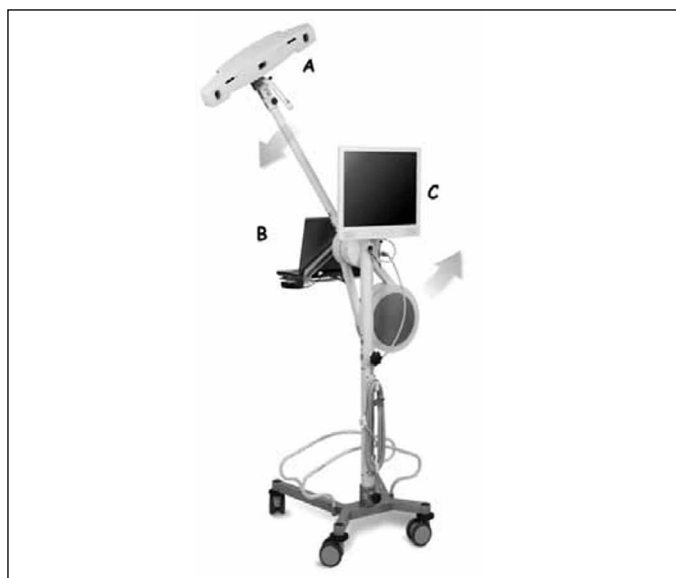
Figure 2 – Navigator with (A) optical tracking camera, (B) computer and (C) monitor.
