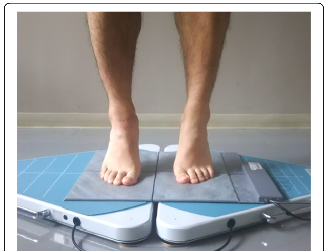
Fig. 4 Measurement of the plantar pressure distribution in the heel-raise position. Participants were kept the maximum heel-raise position for 10 s
