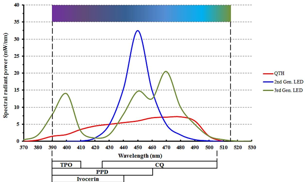
**Figure 1.** Emission spectra from quartz–tungsten halogen (QTH) and light emitting diode (LED) curing lights. The bars underneath show the relationship of the photo-initiators to the LCU spectra. CQ is Camphorquinone, TPO is diphenyl (2,4,6-trimethylbenzoyl) phosphine oxide, and PPD is phenyl-propanedione. (Adapted from Price, 2017 [37]).
