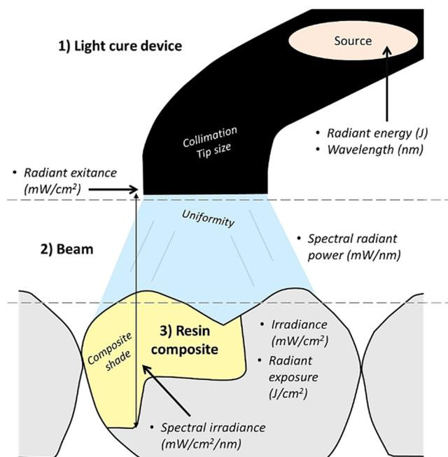
**Figure 3.** A diagrammatic illustration of the process of light curing a resin composite restoration including the relevant terminologies and influencing parameters.
