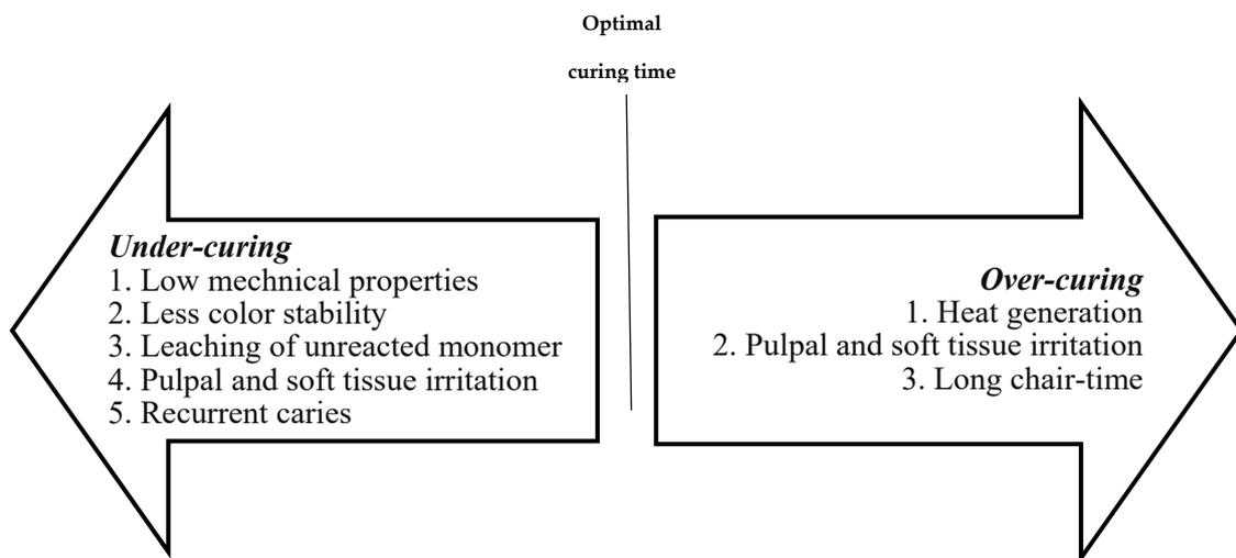
**Figure 4.** A diagram listing the common sequale of under- and over-curing of resin composites.
