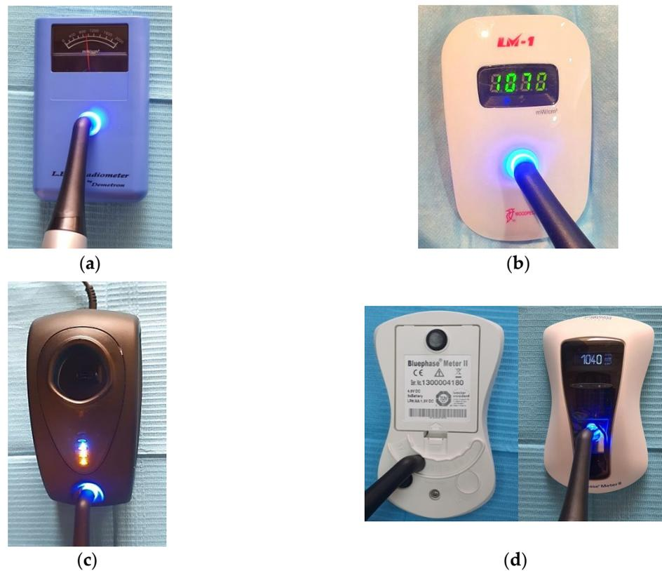
**Figure 6.** Types of dental radiometers: (a) analogue; (b) digital; (c) built into the light cure device's bases, and (d) digital with tip size gauge that influence the irradiance reading.
