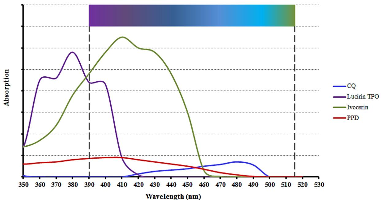
**Figure 2.** Spectral absorption profiles of common photo-initiators found in resin composite formulations. CQ is Camphorquinone, TPO is diphenyl (2,4,6-trimethylbenzoyl) phosphine oxide, and PPD is phenyl-propanedione. (Adapted from Price, 2017 [37]).
