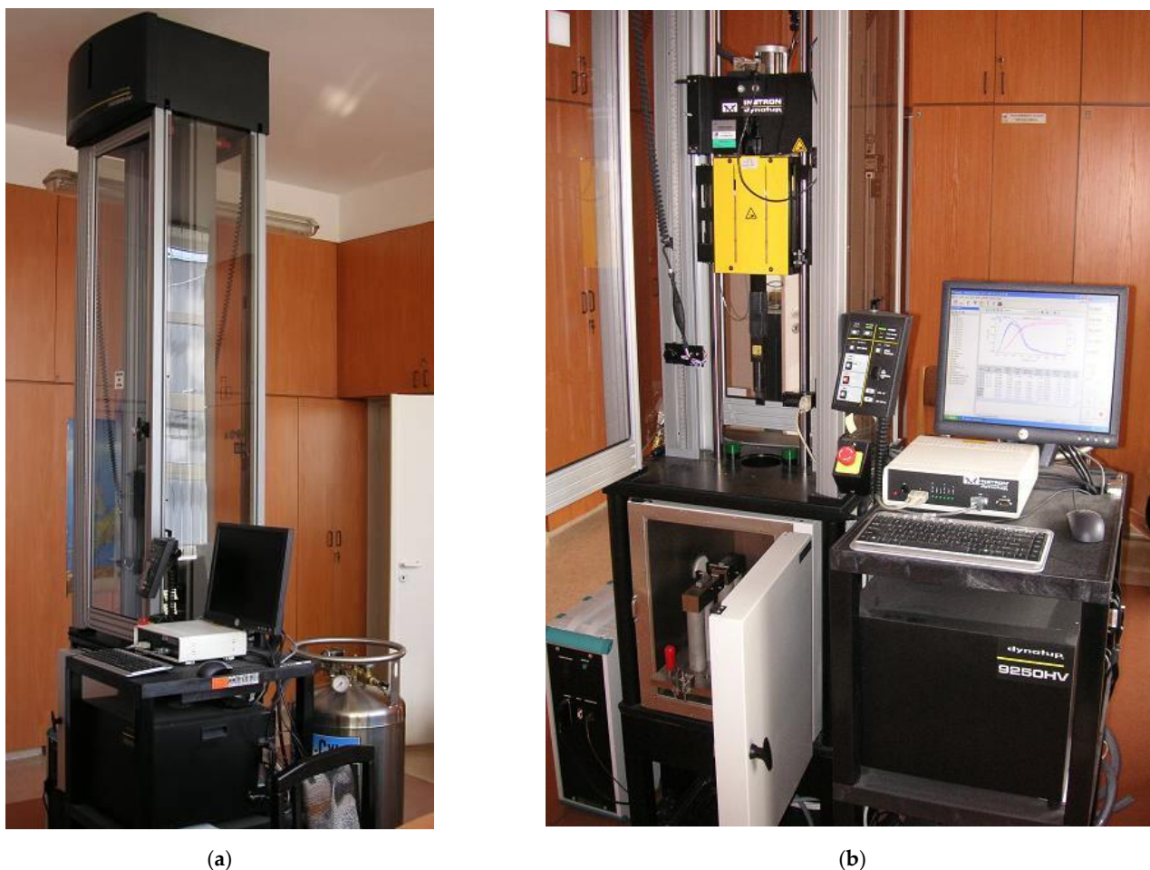
Figure 1. (a,b) Test setup for Charpy impact test.
