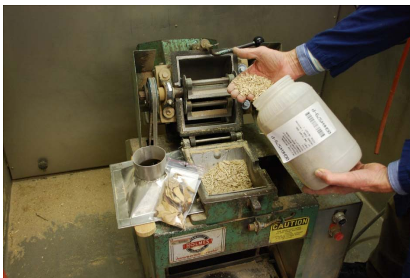
Figure 3. Dry Plant Grinding with a Holmes Hammermill. Note voucher, purpose-built stainless steel funnel, and barcode labeling.
