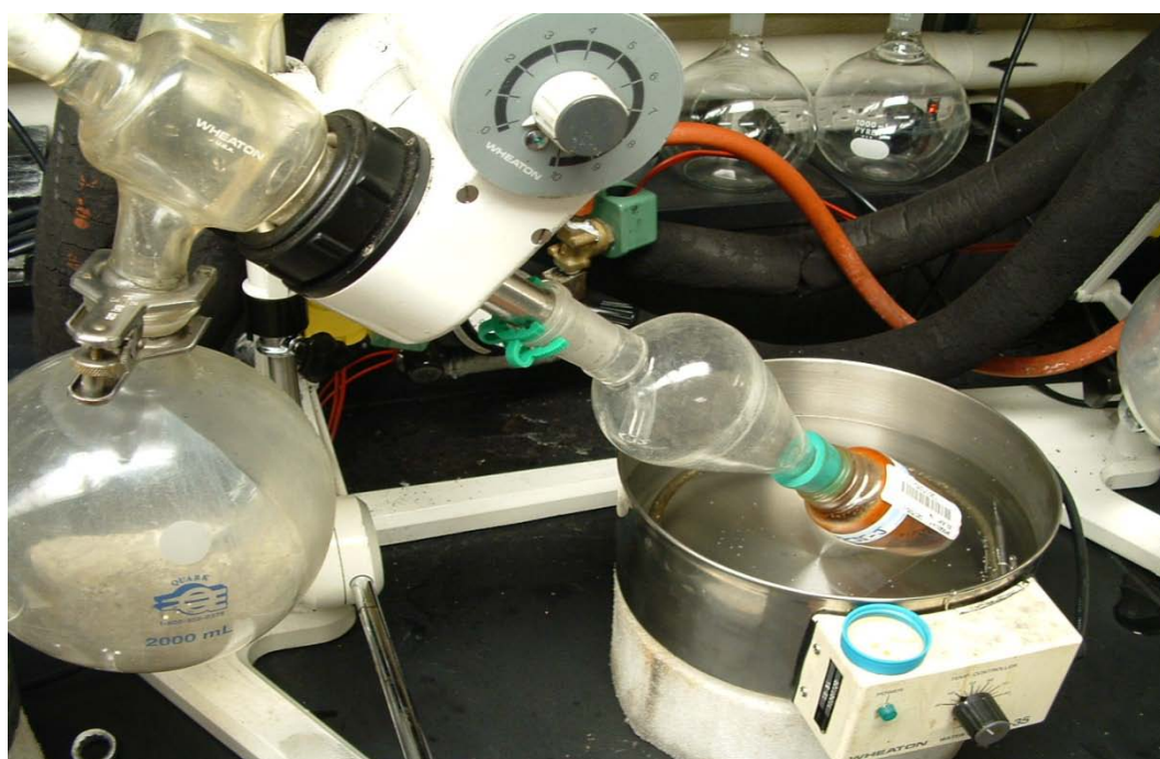
Figure 8. Rotary evaporating to concentrate extract into a bulk storage bottle. Note design of bump trap, Keck clip, Neogreen stopper, vacuum-rated solenoid tied to rotovap rheostat and multiple labeling of the bottle.
