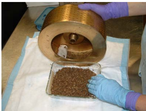
Figure 11. Basket rotor model 1357 with the insoluble marine tissue trapped by paper being removed and transferred into a borosilicate dish for freezing and lyophilization.
