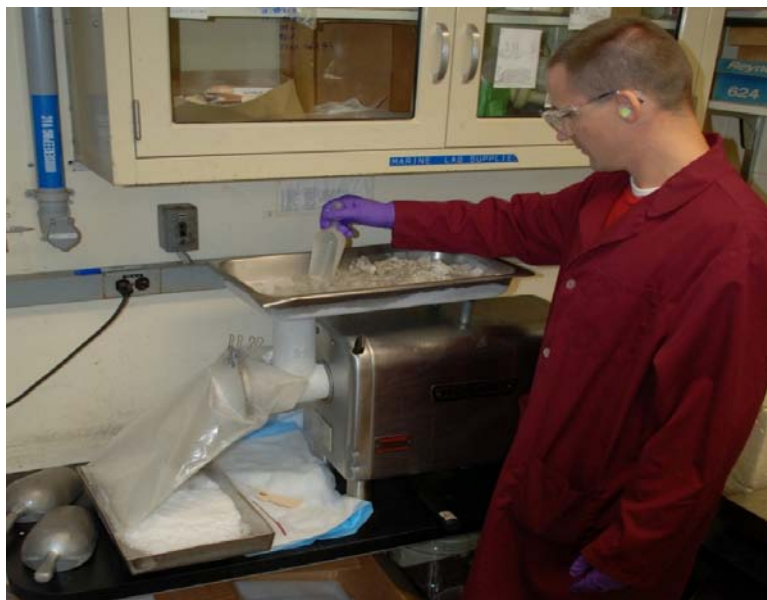
Figure 10. Grinding of marine organism tissue mixed with dry ice.
