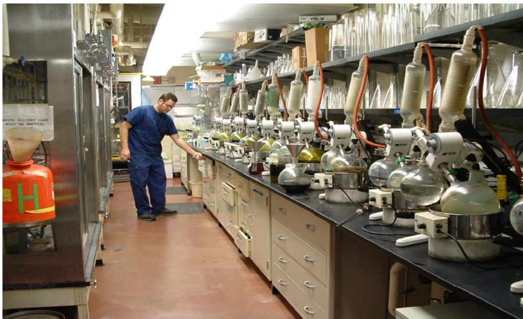
Figure 8. Rotary evaporating to concentrate extract into a bulk storage bottle. Note design of bump trap, Keck clip, Neogreen stopper, vacuum-rated solenoid tied to rotovap rheostat and multiple labeling of the bottle.
