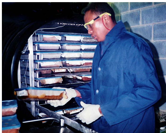
Figure 9. Pyrex dishes containing frozen plant aqueous extracts, capped with paper and a porous lid, are loaded into a VirTis SRC-250 freeze drier.
