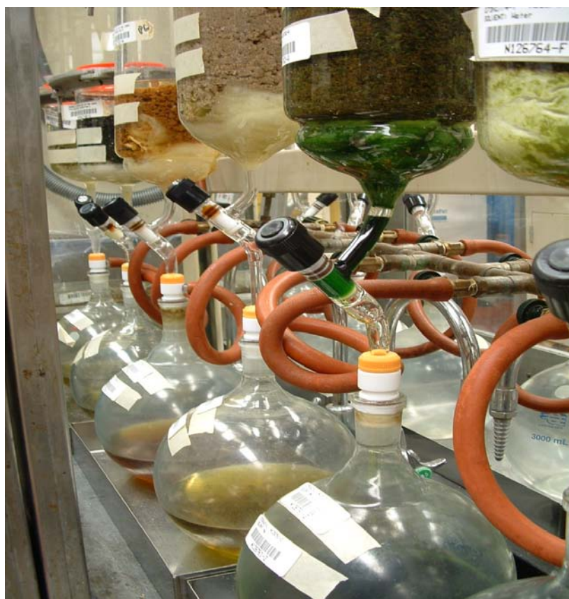
Figure 6. Percolators in use, illustrating bar-encoded labeling over masking tape, cotton filter plug, high vacuum Teflon petcock, vacuum adapter, and 3 L plastic coated flat bottom receiver flask.
