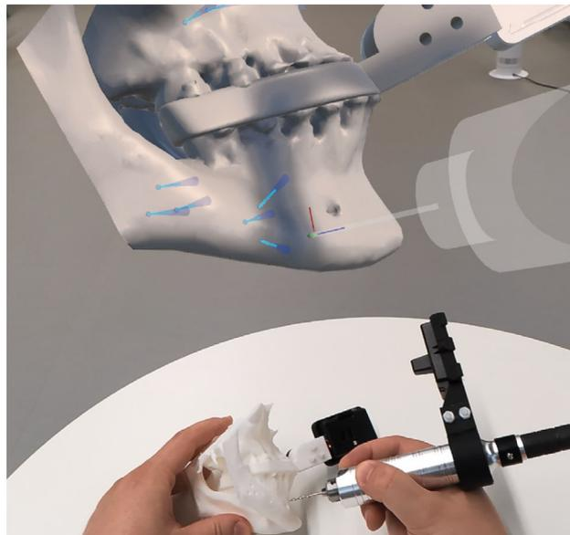
**FIGURE 3** A view from the user perspective using scaled-up 4x 3D holographic model of the VSP with an actively tracked drill using iVation system. Image taken with built-in ML2 screenshot tool.
