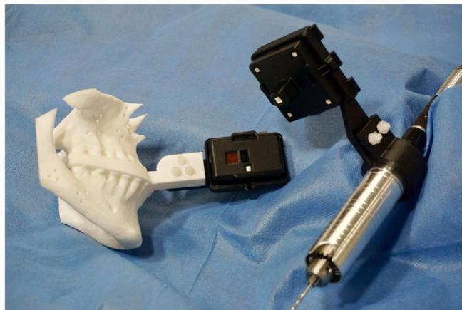
**FIGURE 4** A photograph of the 3D printed skull with the iVation camera attached and the Dremel Drill with the active marker.
