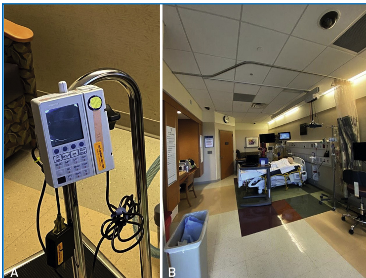
FIGURE 1. Robotic experiment I and the intensive care unit room. A, Intravenous pump device. The objective of the robot was to touch the “Run stop” button, which often alarms when a downstream occlusion occurs. B, Perspective and layout of the intensive care unit room, with the intravenous pump device on the far side behind the bed and near the ventilator.
