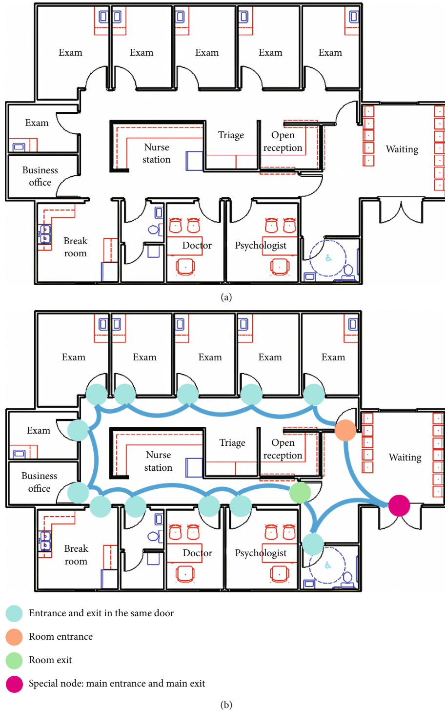
FIGURE 2: A sample of transformation from a floor plan to a graph: (a) the floor plan; (b) the transformed graph.
