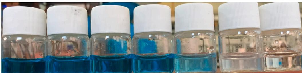
Fig. 8. Sample ( $\text{TiO}_2$ , MB, Air,  $\text{O}_3$ ) after 90 min of exposure.
